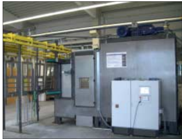
»9 An automatic cleaning system for deplastered and worn-out working moulds
